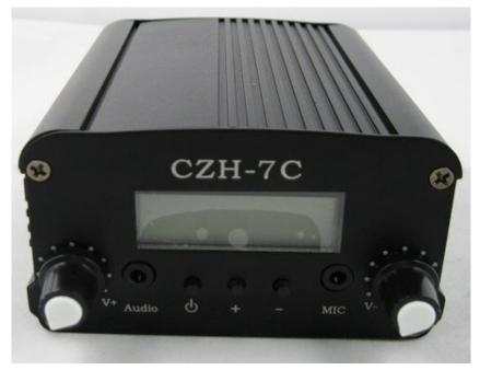
As shown above, for connecting external sound source audio lines connected to "AUDIO" interface. Should use more cable shielding performance audio cable, 3.5mm plug.
